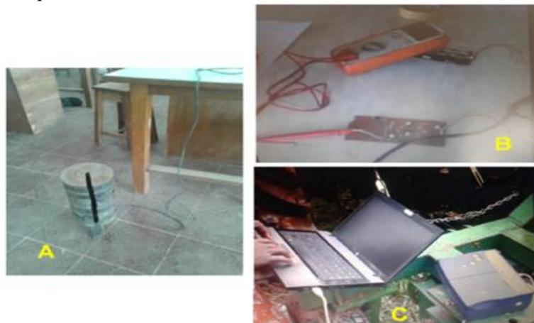
**Figure 1:** Showing (A) Placement of weights on the load cell during calibration, (B) voltmeter and amplifier connecting during load cell calibration and (C) connection of laptop computer to data logger during field test.
