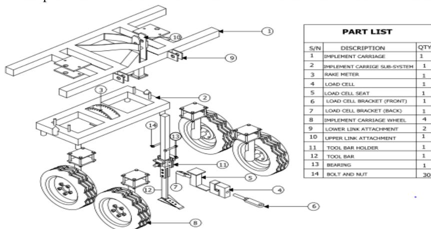
Figure 4: Exploded view of the tool carrier with winged subsoiler and load cell attached
