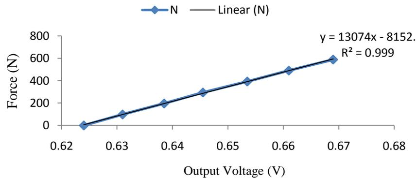
Figure 6: Outpout voltage from instrumentation amplifier due...
