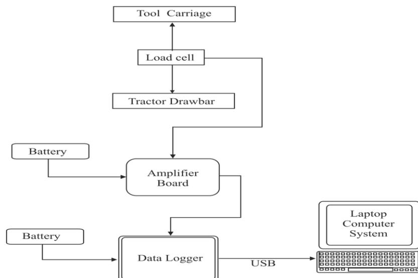
Figure 2: Schematic arrangement of the Instrumentation System for measuring draughts
