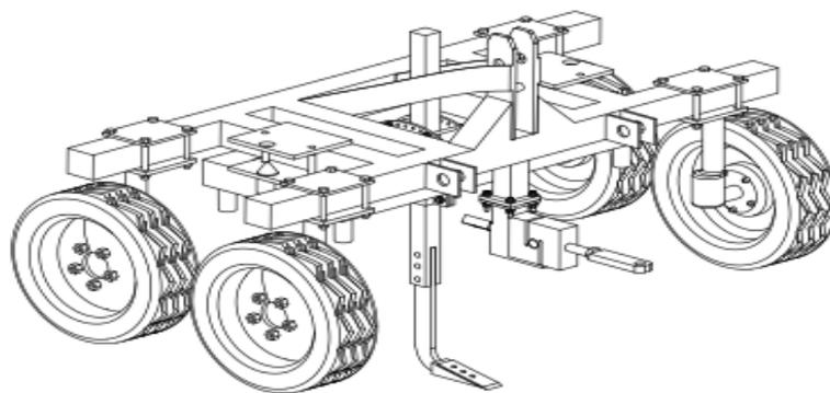
Figure 3: Semi-parabolic subsoiler attached to the tool bar of the carrier with load cell in position
