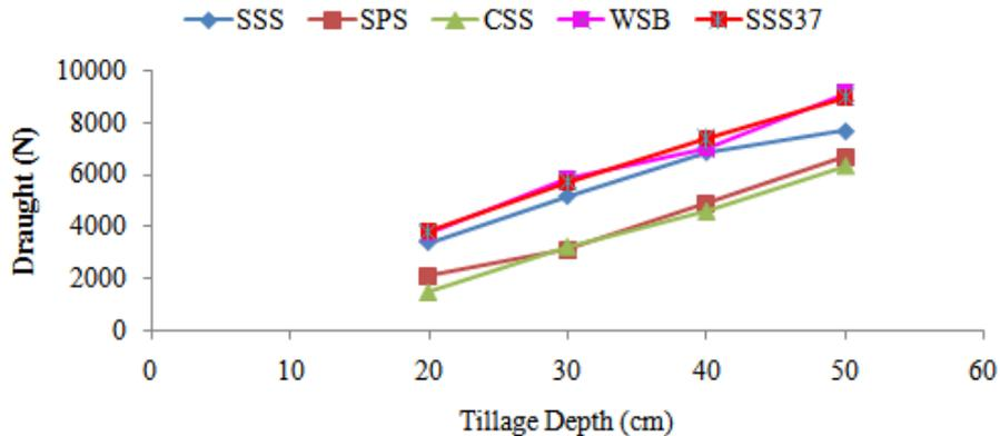
Figure 7: Draught of subsoiler shanks at different depths
